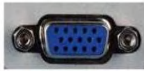
The interface on the graphics card is a 15-pin female connector.
